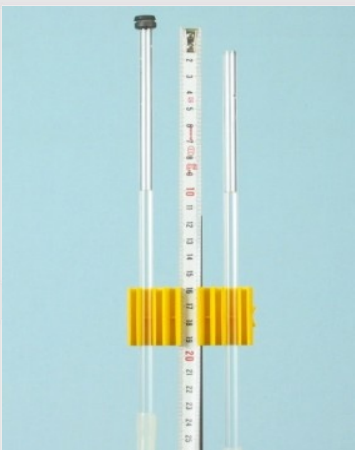
Place the rubber cap on the U-tube
