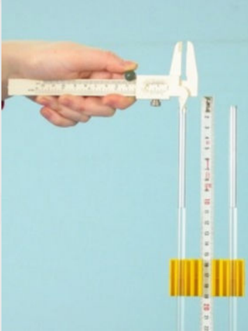
Measuring the inner diameter d_i
