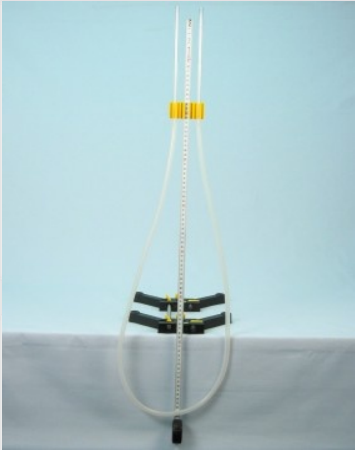
Structure of a U-tube
