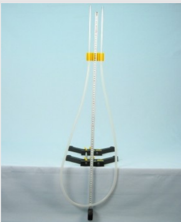
Experimental setup for the investigation of Boyle-Marriote's law
