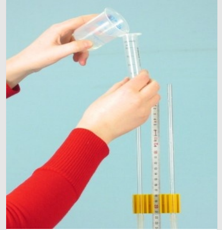
Fill U-pipe with water
